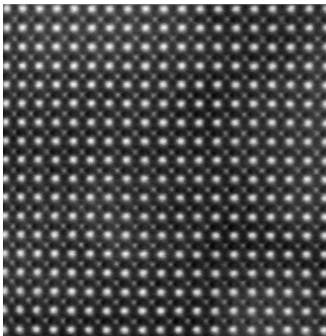
Figure 3.9: STEM-HAADF image of the piezoelectric PZT, with bright Pb columns and darker Zr / Ti columns.
